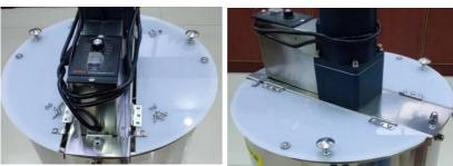
Assemble the two lids with screws.
